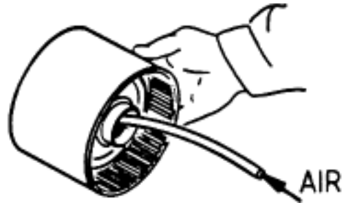
Figure 8.6 Removal of C1, C2 and clutch C4 piston
