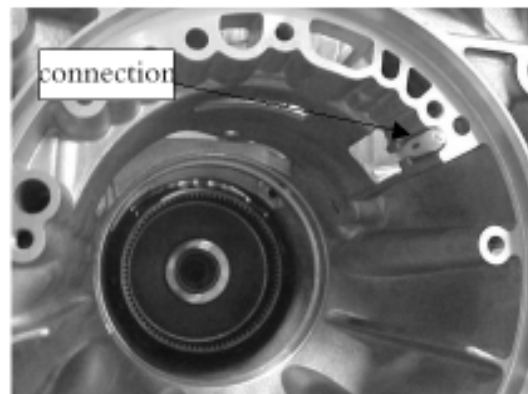
Figure 8.16 Connecting position of coil 7
