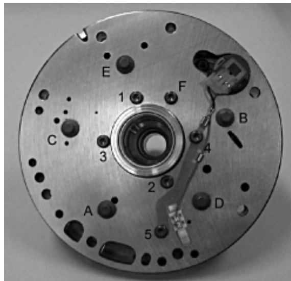
Figure 8.42 Tighten the pump bolt in the sequence shown in figure
