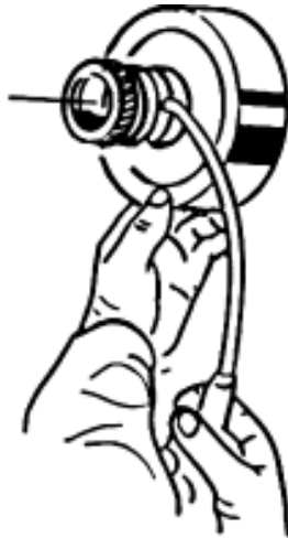
Figure 8.8 Removal of clutch C3 piston
