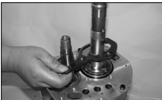
38. Remove the support axial lock plate
