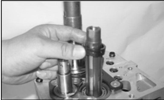
36. Remove the intermediate shaft spacing ring
